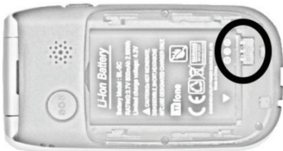
4. Put on the battery cover. Ensure the cover is completely closed and the matching sound (click) could be heard.
